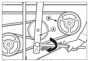
Figure 50. Spindle Drive Belt Removal
